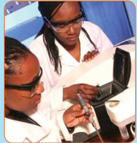
Researchers from the CSIR's drug delivery group measure the size of nano-particles that are used in the Nano-TB drug delivery programme. Photo: CSIR
